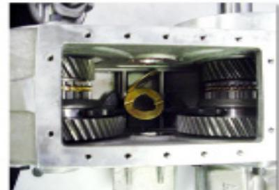
7. Remove the two thrust washers from inside the case.
