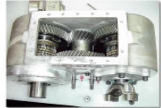
4. Remove the cluster pin retaining bolts.
