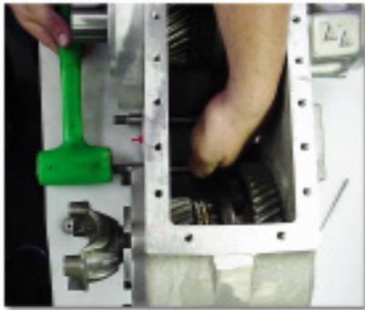
11. Remove the forks from the case. (Note: If you have Atlas case #1929 or earlier and have not upgraded your shifter forks, this is an ideal time to install new shift forks, [P/N 301550](#)).
