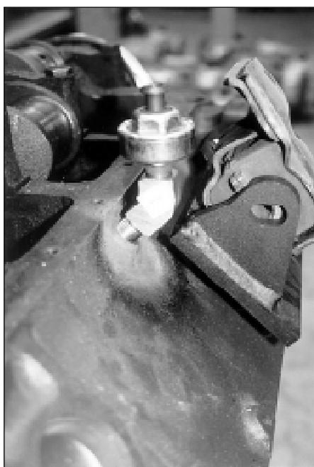
**NOTE:** If you are using a late model block that utilizes an engine block sensor, you will need to purchase a Brass Street Elbow Dorman, Part #490-117. This will allow you to retain your sensor in the original location in order for the block to operate correctly.
