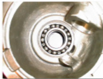
(Fig. 10A) Bearing Installed and Retained with the 716464 Snap Ring
