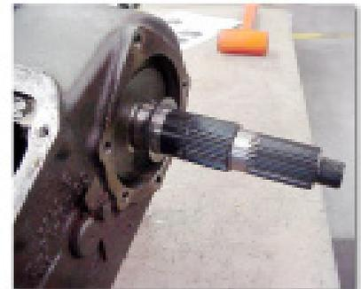
3. Once the gear, shaft, and thrust washer are in place, install the tapered bearing onto the shaft. This should be a light press fit.
