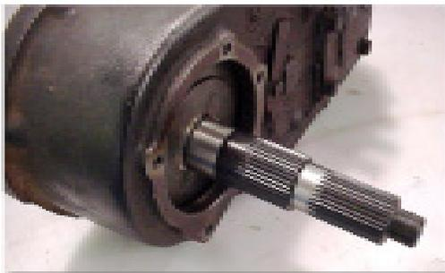
2. Install the shaft through the front of the transfer case, through the slider hub, and onto the stock gear. You should make sure you lube the surface between the gear and shaft. Install the modified thrust washer onto the output shaft. This thrust washer is required to obtain proper gear and slider alignment with the other components in the transfer case.
