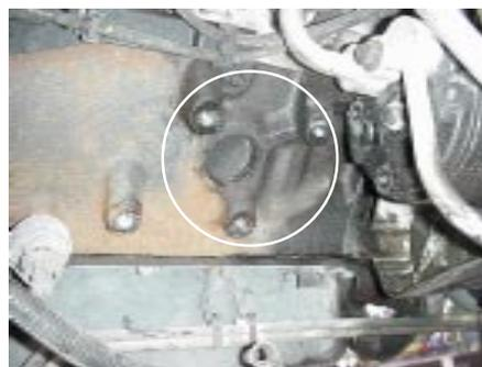
The stock passenger side mount must be removed. The passenger's side LT1 mount used an inverted triangular mount; however, this block also had the standard Chevy mount configuration. The top front hole of the standard mount on this block was used as a support for the air conditioning pump (shown center photo).
