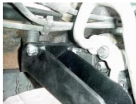
A new bracket has been provided to retain this rear mounting. Mount the new bracket to the air conditioning pump as shown, slip the motor mount between this new air conditioning pump support and the block. Secure the mount and air conditioning pump support to the block with the bolts provided. If you are not planning to retain the A/C and would like to omit this pump, GM offers a bracket and pulley assembly to replace this pump, GM # 10115875.
