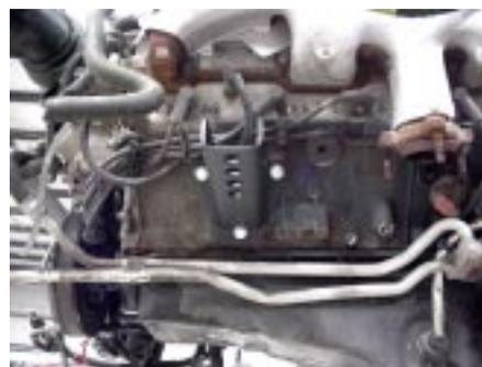
The stock driver's side mount must be removed. The LT1 block has the standard Chevy 3 bolt hole that our conversion mounts bolt to.
