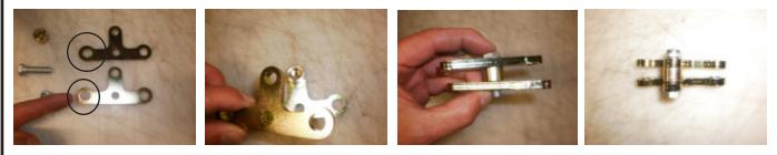
Assemble the shift actuator bracket onto the brass rod end with the slotted portion going on the shift rail closest to the transmission input side of the transfer case.
