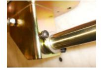
After attachment to cable shifter housing, cycle though all shift points and adjust if shift lever hits the inside of the shifter housing. Install boot retaining ring into supplied shifter boot. Attach shifter housing to vehicle floor using supplied ¼" fasteners. Attach shifter boot to shifter housing using (4) supplied self tapping screws. Install shift knob jam nut and shift knob.
