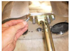
The new brass shift rail ends need to be threaded onto the shift rails. The Igus bushings should be install prior to threading them to the shift rails. Install the brass completely onto the shift rail and then back it off two complete turns, the Igus bushing to be located towards the top of the transfer case.
