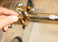
Loosely assemble supplied heim onto the 5/16"-24 cable threads. NOTE: The cable only mounts to the transfer case in one direction. Inspect the cable and find the end with a grove on in. The opposite end has a threaded section for mounting to the handle. Connect the groved end to the Heim joint. Attach the cable onto cable mounting bracket with supply U-bolt and 5/16"-24 thin locknuts.
