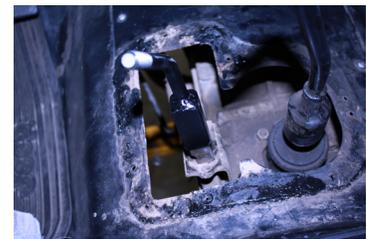
The stock shifter will need the four edges chamfered since the new handle with the tube fitting over this section has radius corners. Grind the edges and then test fit until the handle slides all the way on. The handle is an exact fit with no bushings, just a set screw to lock in place. The handle comes with a new shifter knob that is laser etched with the NP231 shift pattern.
