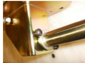
After attachment to cable shifter housing, cycle through all shift points and adjust if shift lever hits the inside of the shifter housing. Install boot retaining ring into supplied shifter boot. Attach shifter housing to vehicle floor using supplied 1/4" fasteners. Attach shifter boot to shifter housing using (4) supplied self tapping screws. Install shift knob jam nut and shift knob.
