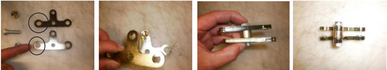
Assemble the shift actuator bracket onto the brass rod end with the slotted portion going on the shift rail closest to the transmission input side of the transfer case.
