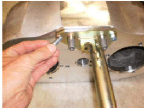
The new brass shift rail ends need to be threaded onto the shift rails. The Iglas bushings should be install prior to threading them to the shift rails. Install the brass completely onto the shift rail and then back it off two complete turns, the Iglas bushing to be located towards the top of the transfer case.
