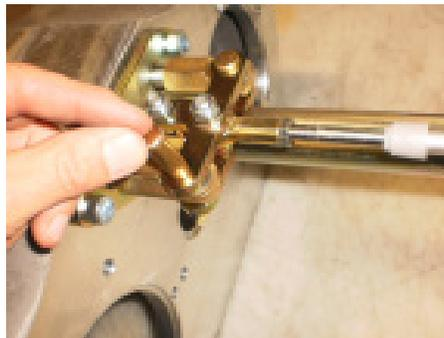
Loosely assemble supplied heim onto the 5/16"-24 cable threads. NOTE: The cable only mounts to the transfer case in one direction. Inspect the cable and find the end with a groove on in. The opposite end has a threaded section for mounting to the handle. Connect the groved end to the Heim joint. Attach the cable onto cable mounting bracket with supply U-bolt and 5/16"-24 thin locknuts.
