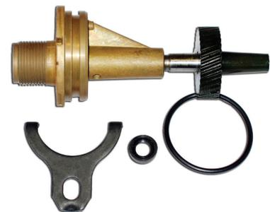
This tailhousing offers a speedometer option (sold separately). This tailhousing is designed to fit a stock Jeep (1983-86) mechanical driven speedometer housing. Vehicles requiring a cable connection for the speedometer can order [P/N 301506](#). The speedometer gear is not included with this housing, but by using the charts above you can select the correct gear for your tire size and axle ratio.
