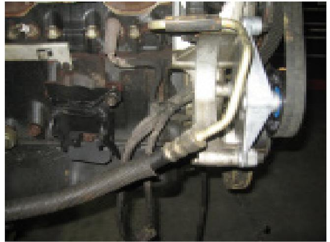
The LT1 engine can be used with the bolt in YJ mount as long as you replace the A/C pump with the Chevy P/N 10115875. This is a replacement pulley for the LT1 that removes the A/C pump. The replacement pulley is slightly smaller in diameter and will require a new belt.
